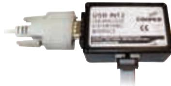
TTL to RS232 - Wireless survey tool connection (serial link)
