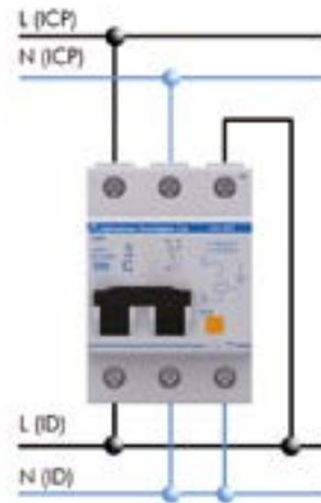
**IGA TEST** protectors actuate when they detect a permanent overvoltage (for example, a fault in the neutral), protecting the equipment installed downstream.
