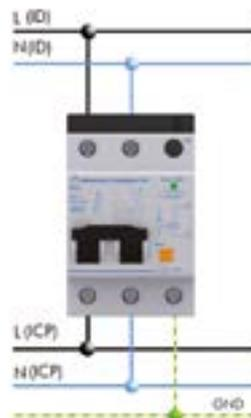
IGA TEST COMPACT protectors cut off the power supply when they detect a permanent overvoltage, (for example, a fault in the neutral), thus protecting the equipment installed downstream.
