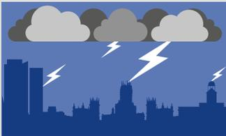
One of these objects will be the one forming the upward leader, which will move towards the downward leader thus forming the discharge path between the cloud and the ground. This object will receive the lightning strike. The cloud charge will find the most direct path to earth. If this path is not controlled, it could cause serious damage.
