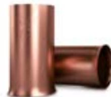
**AT-072NCXX:** Copper adapter sleeves with variable diameters depending on XX selection. XX indicates the mm<sup>2</sup> of the desired cable. They increase the conductor diameter fitting it in a mould designed for this XX bigger cable. X = 50, 70, 120...
