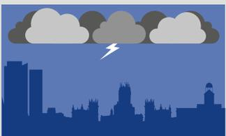
When the electric field is high enough, the cloud starts discharging towards the ground. The path formed by this discharge is called the downward leader and produces a very sharp variation in the electric field which affects the positive charges in the objects on the ground, causing the corona effect.
